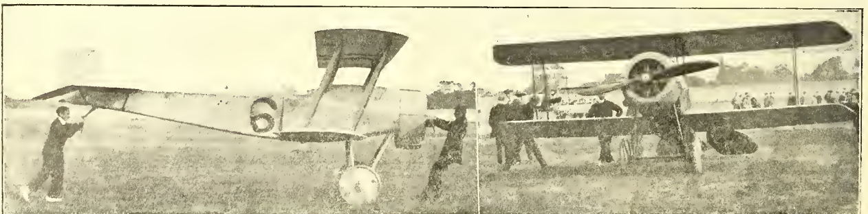
Lord Carbery's Bristol Scout, as it now appears with an 80-h.p. Le Rhône engine.
